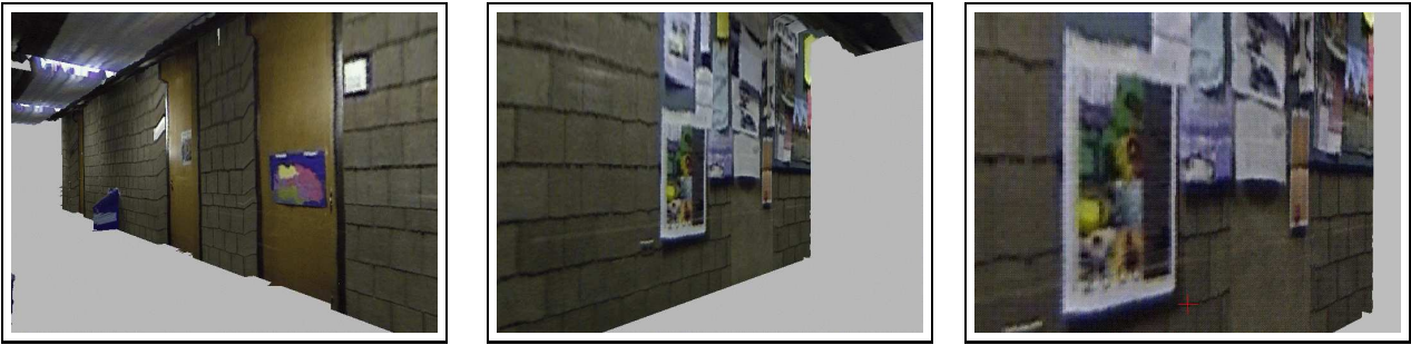
Figure 3. 3D Model generated (a) from raw sensor data, and (b) using our algorithm, in which 94.6% of all measurements are explained by 7 surfaces. Notice that the model in (b) is much smoother and appears more accurate.
