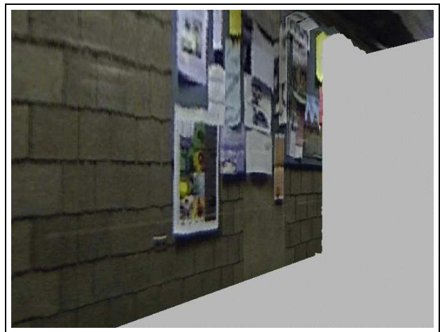
Figure 3: 3D Model generated (a) from raw sensor data, and (b) using our algorithm, in which 94.6% of all measurements are explained by 7 surfaces. Notice that the model in (b) is much smoother and appears more accurate.
