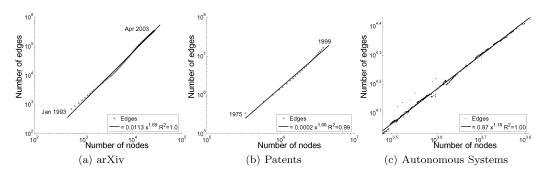
**Fig. 5.** The Densification Power Law. The number of edges E(t) is plotted against the number of nodes N(t) on log-log scales for (a) the arXiv citation graph, (b) the patents citation graph, and (c) the Internet Autonomous Systems graph. All of these grow over time, and the growth follows a power law in all three cases [Leskovec et al. 2005].
