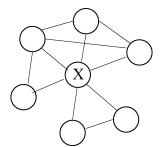
**Fig. 3.** Clustering coefficient. Node X has  $k_X = 6$  neighbors. There are only  $n_X = 5$  edges between the neighbors. So, the local clustering coefficient of node X is  $n_X/k_X = 5/15 = 1/3$ .
