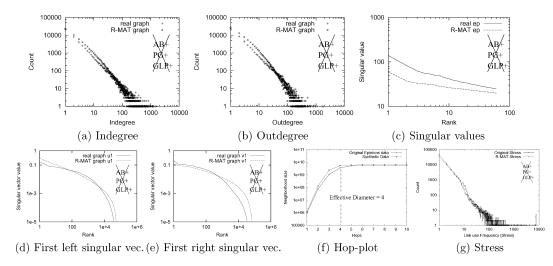
**Fig. 17**. Epinions directed graph. The *AB*+, *PG*+ and *GLP*+ methods **do not apply**. The crosses and dashed lines represent the R-MAT generated graphs, while the pluses and strong lines represent the real graph.
