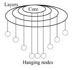
Fig. 6. The Internet as a Jellyfish. The Internet AS-level graph can be thought of as a core, surrounded by concentric layers around the core. There are many onedegree nodes that hang off the core and each of the layers.
